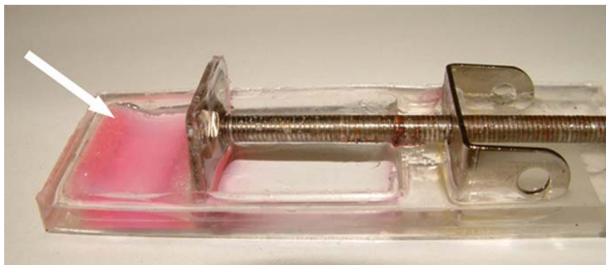
Fig. 14.5 Uniaxial loading device. The FCM (pink) is connected to parallel walls via Velcro ® rods (white arrow), where the left wall was fixed and the right wall can be pulled to the right. The FCM was strained by at maximum 5% after gelation (3T3 fibroblasts were labelled with cytoplasmic fluorescent dye and added to the gel at a final concentration of 1 \times 10^5 cells/ml)
